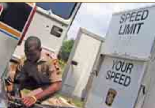
Cadet Reginald Forbes helps set up the Agency's speed trailer, which displays the speed of passing vehicles.
