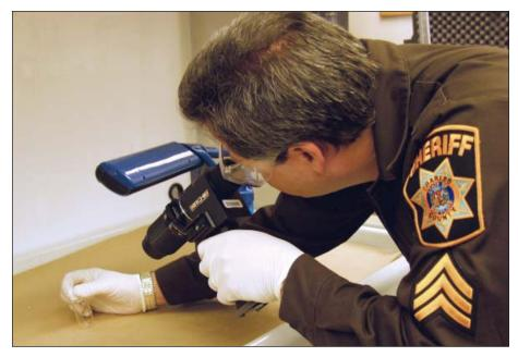
Sgt. Joseph Goldsmith scans evidence for fingerprints with a reflective ultra-violent imaging system. Ultra-violet light travels through filters in the equipment and will illuminate fingerprints in daylight without the need for technicians to pre-process the prints.
